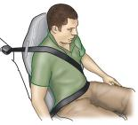
If it is necessary for an occupant to adjust their seat or seating position during a journey, the belt tension might be disturbed. The occupant should therefore (as soon as it is safe to do so) gently pull down the shoulder run of the seat belt to create some slack and then immediately release it to re-tension the belt for the new seating position.
