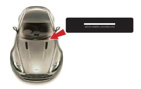
The Vehicle Identification Plate, attached to the right hand suspension strut tower, is model and market dependant.
