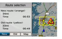
If the system calculates an alternate route, the new route is shown in orange while the old route is shown in yellow. Information is also given on the overall length of both routes as well as the estimated travel time to the destination.
