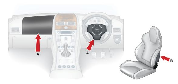
The vehicle is equipped with driver and passenger airbags. The airbags and seat belt pretensioners (Refer to 'Pre-tensioner and Load Limiting Systems', page 3.9) are electrically controlled by an advanced restraints system.
