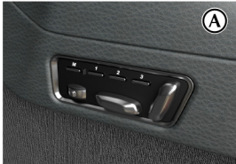
The memory function buttons are located in the seat adjustment controls which are located each side of the centre console (A).
